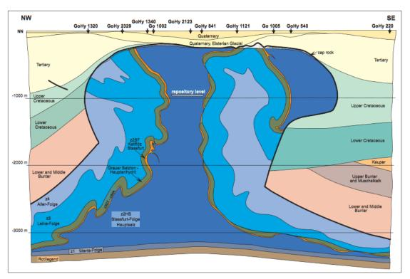
Figure 41: Simplified cross section of the Gorleben salt dome (modified according to Bornemann 1991)
